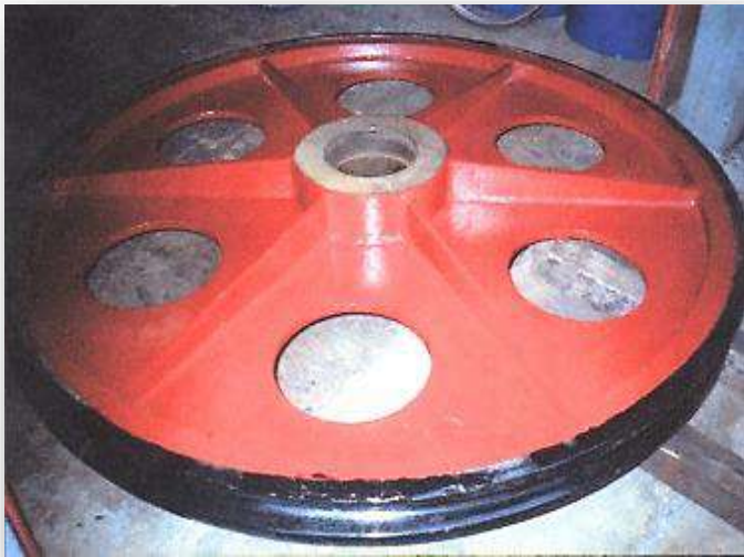
Philex Mining Corp., Pulley Groove 800ø Polyurethane
