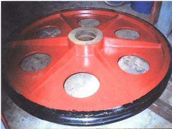
Philex Mining Corp., Pulley Groove 800ø Polyurethane
